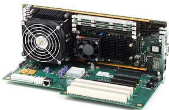
Figura 20. PICMG 1.3 Single Board Computer (SHB) en un Backplane activo.
